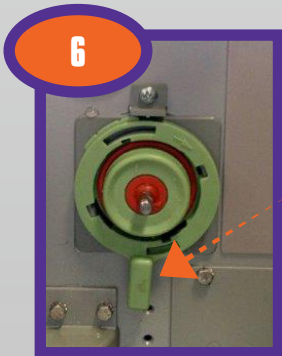
6 Rotate green locking lever anti-clockwise (6 o'clock position)
