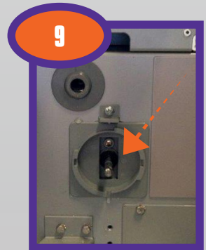
9 Clean motor assembly and machine body.
