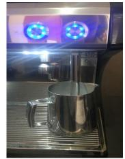
• Press the barista steam button again, it will automatically go through the cleaning cycle again and stop when finished.
