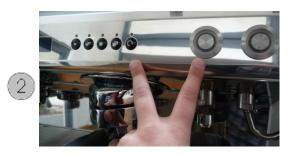
Start the cleaning cycle by pressing and holding the button T5 right of the keyboard and the button on the B.S. (push button T5 first). The cycle starts automatically after 3 seconds.
