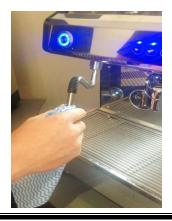
If the wand becomes blocked (no steam when you open the tap), despite taking meticulous care with cleaning. Dismount the diffuser and then clean it.
