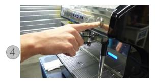
Start again the cleaning cycle by pressing the B. S. button. Wait the end of the cycle (about 1 minute). The end is indicated by the buzzer and the indication on the display.
