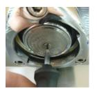
With a screwdriver, remove the shower and the shower holder. Put these two elements in a container which contains water and two detergent tablets (*ref 9003479*). Leave it overnight and clean these parts with a brush to remove all grease of coffee and assemble them back on the brewhead.
