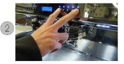
Connect the filter-holder. Hold down both buttons simultaneously on the ends to start the cleaning cycle. The LEDs flash from left to right.
