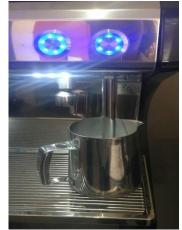
Start the cleaning cycle by holding down the continuous dose button on the RHS keypad and the barista steam button. The cycle starts automatically after 3 seconds.
