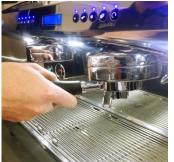
Hold down both buttons simultaneously on the ends of the desired group to start the cleaning cycle. The LED's will flash from left to right.
