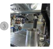
After about 2 minutes the cleaning cycle stops (indicated by the buzzer). Fill the pitcher and rinse it with water (maximum temperature: 25 ° C) Place the pitcher under the B.S. with the lance submerged in water.
