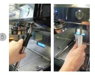
Remove by unscrewing the stainless steel part and clean the arm with a damp cloth.
