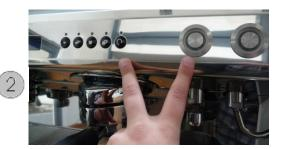
Start the cleaning cycle by pressing the button T5 right of the keyboard and the button on the B.S. (push button T5 first). The cycle starts automatically after 3 seconds.
