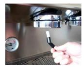
Disconnect the filter-holder and perform the cleaning operation on the joint of the brewhead, using the brush.
